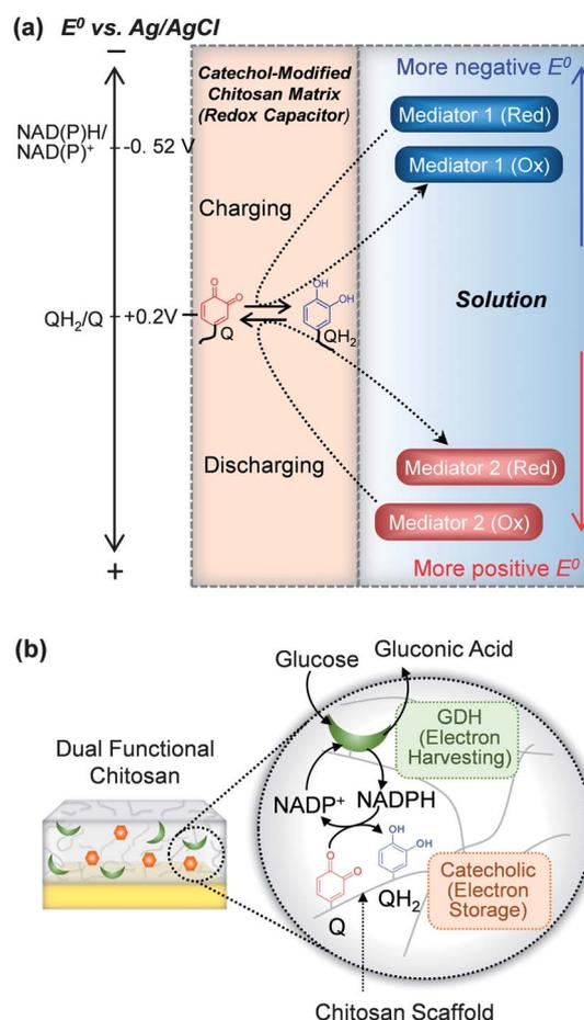
**Fig. 7** Tyrosinase-catalyzed grafting of catecholic natural products confers redox properties. (a) Schematic illustrating the redox-capacitor capabilities of the catechol-modified film; the film can accept, store and donate the electrons. (b) A dual functional film uses glucose dehydrogenase (GDH) to harvest electrons from glucose and transfer them to the film by an NADPH redox-cycling mechanism.
