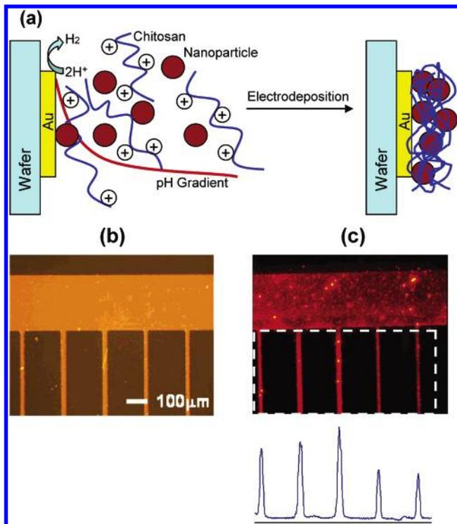
**Figure 4.** Chitosan's electrodeposition can mediate nanoparticle assembly. (a) Mechanism of chitosan-mediated nanoparticle deposition at the cathode. (b) Photomicrograph of silicon wafer patterned with 20  $\mu\text{m}$  gold lines that were biased for deposition. (c) Fluorescence photomicrograph showing spatially localized deposition of 100 nm fluorescent latex spheres from a 1% chitosan solution (pH = 5).<sup>55</sup>
