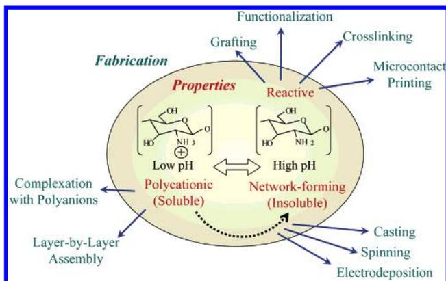
**Figure 1.** Schematic illustrating chitosan's versatility for fabrication. At low pH (less than about 6), chitosan's amines are protonated conferring polycationic behavior to chitosan. At higher pH (above about 6.5), chitosan's amines are deprotonated and reactive. Also at higher pH, chitosan can undergo interpolymer associations that can lead to fiber and network (i.e., film and gel) formation.
