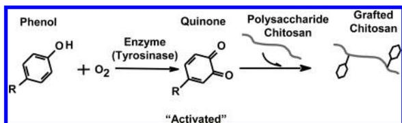
**Conjugation: Enzymatic Assembly of Proteins onto Chitosan.** Figure 5 shows two important features of the tyrosinase-initiated grafting to chitosan. The scheme in Figure 5a illustrates that tyrosinase's substrate range is not limited to low molecular weight phenols, but rather this enzyme can oxidize accessible tyrosine residues of proteins. Thus, tyrosinase serves to “activate” proteins for their assembly (i.e., conjugation) onto chitosan.<sup>115</sup>
