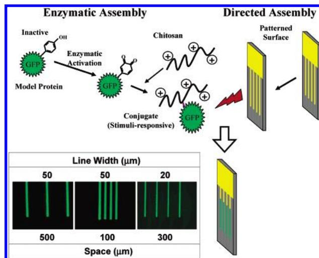
**Figure 6.** Coupling directed assembly with enzymatic assembly to selectively assemble a protein at a microfabricated address. Schematic showing that conjugation requires enzymatic activation, electrodeposition requires an imposed electrical signal, both provide added control to protein assembly. Fluorescence photomicrographs show the assembly of the GFP–chitosan conjugates onto micropatterned cathodes of varying sizes and spacing.
