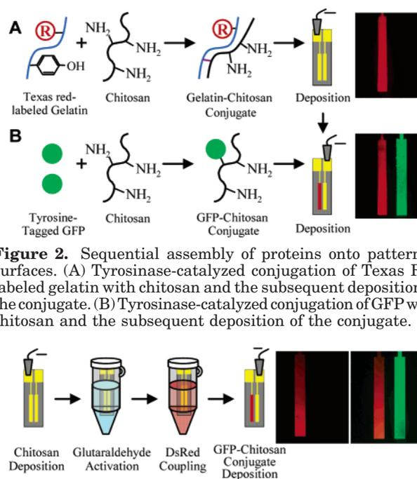
**Figure 2.** Sequential assembly of proteins onto patterned surfaces. (A) Tyrosinase-catalyzed conjugation of Texas Red labeled gelatin with chitosan and the subsequent deposition of the conjugate. (B) Tyrosinase-catalyzed conjugation of GFP with chitosan and the subsequent deposition of the conjugate.
