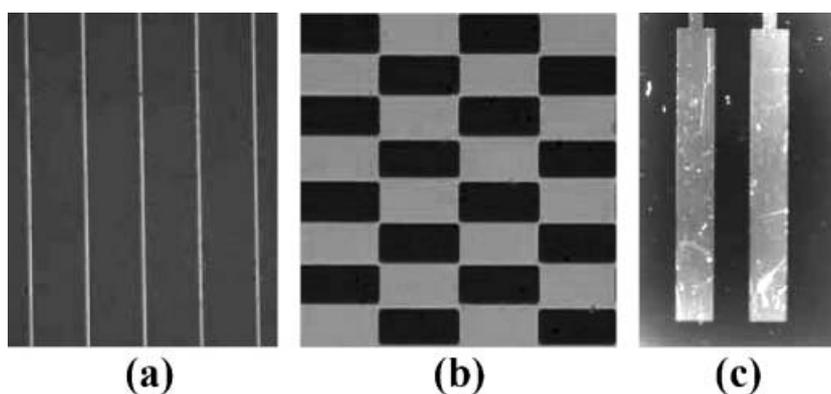
**Figure 1.** Photomicrographs of patterned chips used in this study: (a) parallel gold lines (20 μm wide lines separated by 500 μm spaces) that are connected to a single lead; (b) grid of interconnected gold rectangles (200 μm × 360 μm) that are connected to a single lead; (c) chip with two gold rectangular electrodes (8 mm × 1 mm) that are connected to separate leads (i.e., the electrodes are electrically independent).
