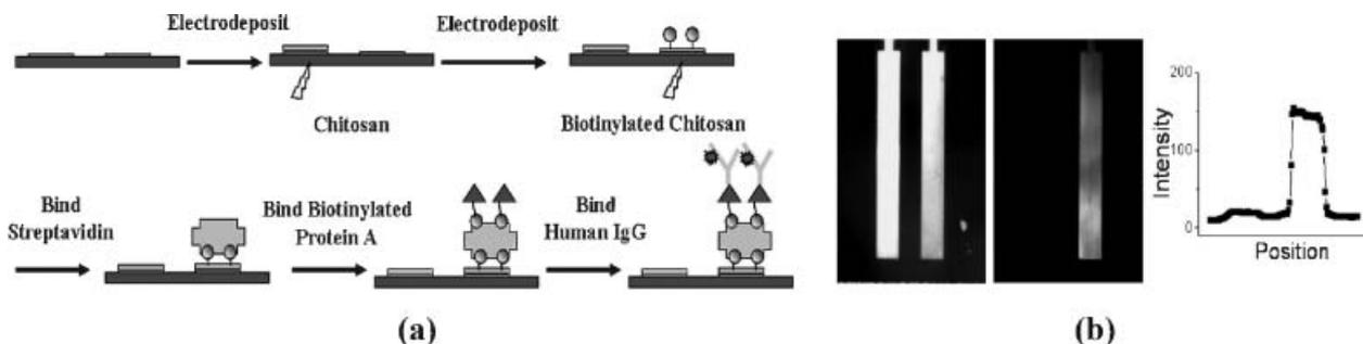
**Figure 4.** Streptavidin-mediated protein assembly: (a) schematic of experiment; (b) bright-field photomicrograph and fluorescence photomicrograph with fluorescence intensity profile showing fluorescently labeled IgG is assembled onto the right electrode (with biotinylated chitosan) with little non-specific assembly on the left electrode (with chitosan).
