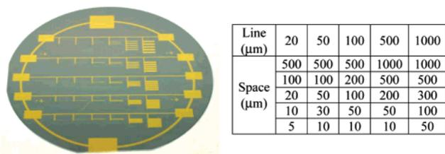
**Figure 2.** Photograph of a patterned surface with gold lines of varying widths and varying spaces. The table next to the photograph lists the widths of the gold lines and the spaces.
